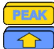
*During the measurement, if pressed for a second, it activates the PEAK+ function, (it displays the greatest force detected after having activated the function).*
