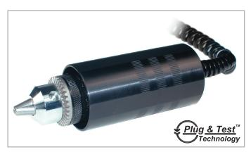
Series R50 smart sensors measure bi-directional torque for a wide variety of applications across virtually all industries. Contain a Jacobs chuck for up to 0.5 in [12.7 mm] diameter samples, bits, or fixtures. The sensors can be used as hand held devices, or mounted to a test stand. Capacities available from 10 ozFin to 100 lbFin [7 to 1150 Ncm]. Compatible with Mark-10 model 5i and 3i indicators (sold separately) through unique Plug & Test™ technology.
