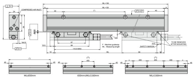
(\*) Add holes at 40mm from cut ends, when the first hole at constant step is at a distance X>175mm.
