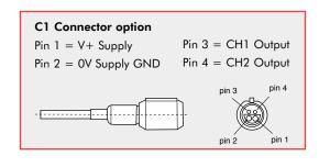
When connecting the sensor, care should be taken with the correct connections. The sensor is provided with reverse polarity protection and short circuit protection between outputs (Yellow & White) to GND (Black), but if the outputs (Yellow & White) are connected to the supply this will result in device failure.
