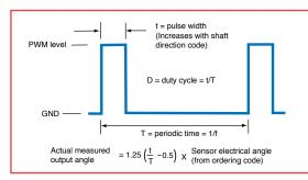
PWM levels = zero volt and 5V ( $\pm$ 3%) for 9-30V supply = zero volt and V<sub>s</sub> ( $\pm$ 1%) for 5V supply
